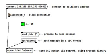
Figure 4. Microphone control via OSC.
