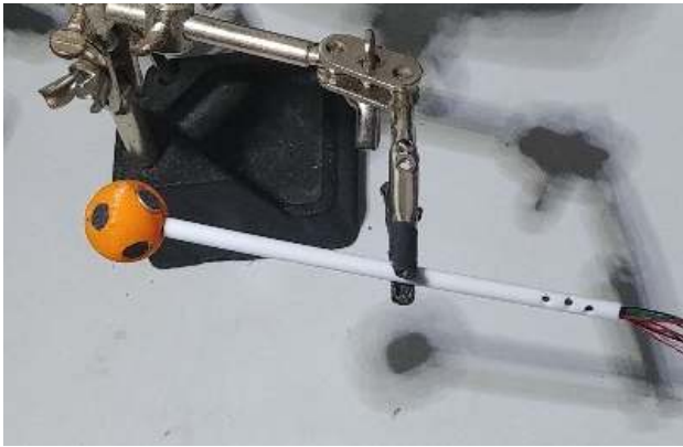
Figure 7: A 3D microphone array prototype with 6 orthogonal capsule
