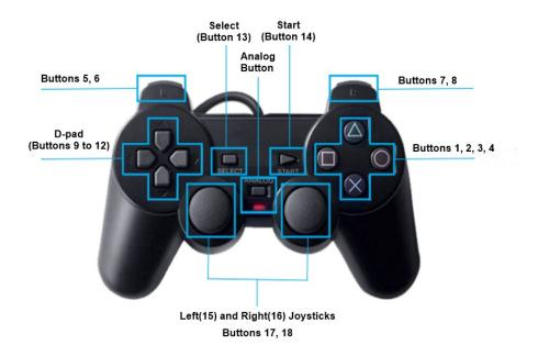
Figure 1: Joystick controls used in this work
