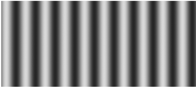
Figure 7. A 8-bit wave file of a 441Hz sinusoid lasting 10 seconds in 44100Hz mapped to a image with 1000 pixels of width.
