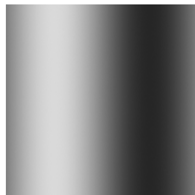
Figure 6. A 8-bit wave file of a 210Hz sinusoid lasting 1 second in 44100Hz mapped to a image with 210 pixels of width.
